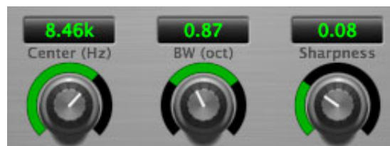
Figure 21.2: Ess Band Filter Controls
