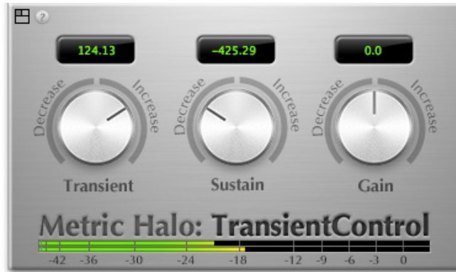
Figure 23.4: Basic: Provides the Minimum Controls and Metering
