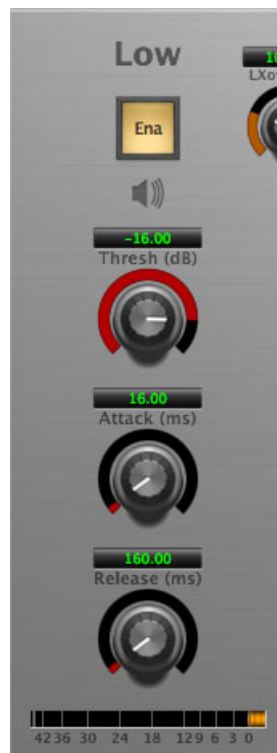
Figure 5.4: Expander (Low Frequency Shown)
